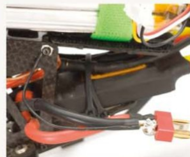
Allow static electricity to discharge to ground rather than build up in the frame.
