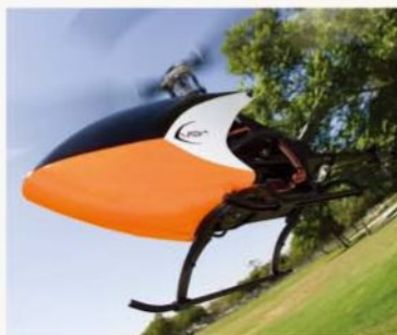
The carbon infused frames on the Protos allow static to discharge.
