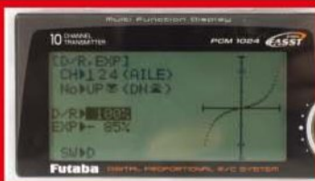
As you can see in the graph above, expo lowers the sensitivity of the stick as you get closer to the center without affecting total available throw.
